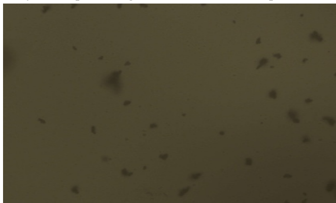
Figure 4. OM Image of ZnO Nanoparticles
